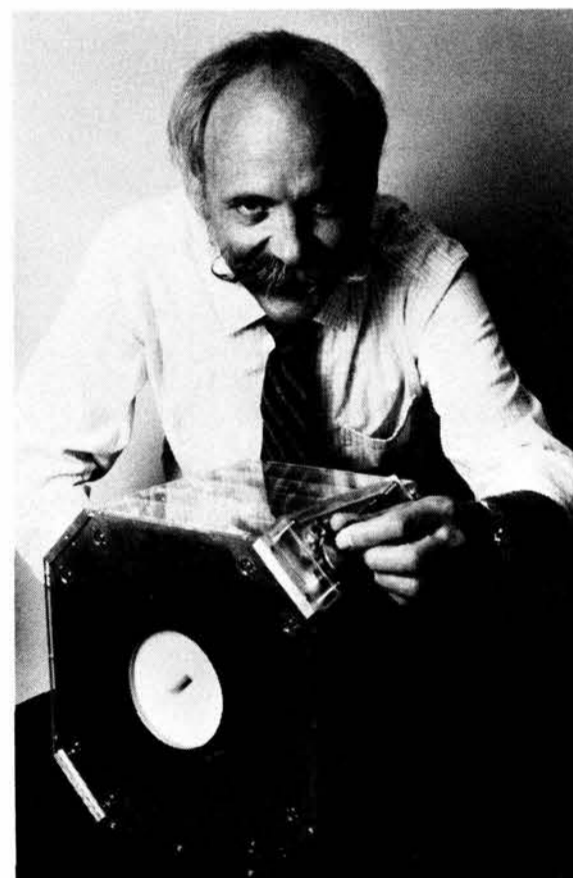
INVENTOR RON HILL (2561) displays a prototype model of his variable aperture neutron collimator that was recently patented. The mechanical device provides an adjustable-size square or rectangular aperture in a uniformly diverging line-of-sight from a neutron source. The device would be used with a neutron generator for medical applications.
